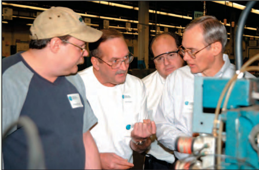
At General Cable's plant in Altoona, Pennsylvania, (l-r) associates Gregg Mazak, electro-mechanic, and Jim Porter, production manager, explain to Roger Roundhouse, vice president, automotive, and Larry Fast, senior vice president, operations, the Six Sigma-initiated modifications they made to the Artos machines to reduce scrap in the ignition wire manufacturing process. Photo courtesy of General Cable Corporation.
